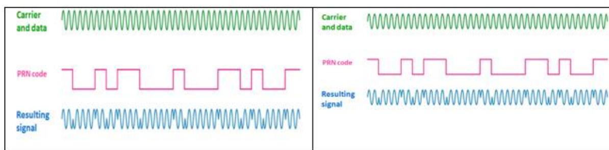
Figure (5). GPS signal model
