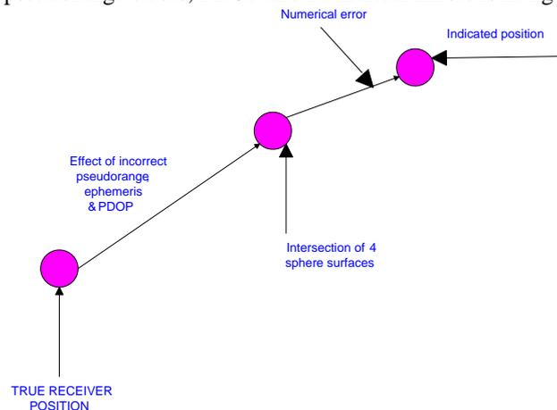
**Figure 11.** Pseudorange errors, PDOP and Numerical Errors
