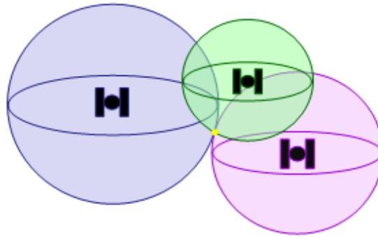
Figure 7(b). Three satellites (2-D) Positioning model
