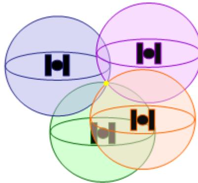
Figure7(c). Four satellites (3-D) Positioning model
